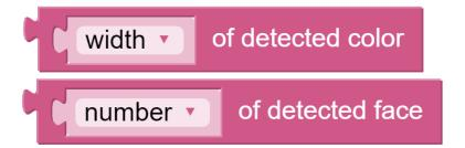
These two blocks are used to output information. The detection result has five output values, namely coordinate x value, coordinate y value, width, height, and number.
