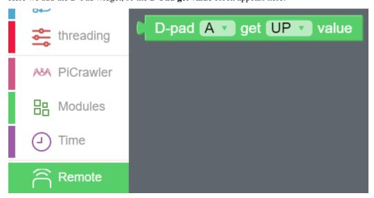
D-Pad can be regarded as a four-in-one button. You can choose which button to read in the second groove of the block. When the button is pressed, the value is "1"; when the button is not pressed, the value is "0".
