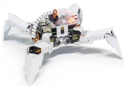
PiCrawler is a Raspberry Pi quadruped robot with aluminum alloy structure. It is equipped with a camera module, which can perform color recognition, face detection and other items; 12 metal gear servos support it to walk, dance, and pose various postures; the ultrasonic module on the body allows it to quickly detect obstacles in front of it; the expansion board-robot HAT is equipped with a speaker, allowing it to express emotions such as happiness and excitement.
