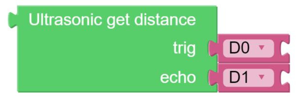
It should be noted that the two pins of the block should correspond to the actual wiring, that is, trig-D2, echo-D3. Here is the main program.
