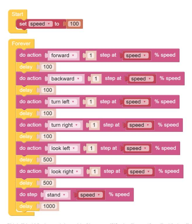
Click the Upload & Run button at the bottom right of the screen, and PiCrawler will execute "forward" and "backward" actions in sequence.
